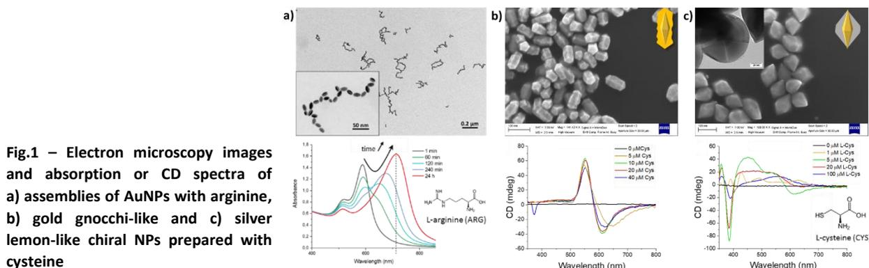
Fig.1 – Electron microscopy images and absorption or CD spectra of a) assemblies of AuNPs with arginine, b) gold gnocchi-like and c) silver lemon-like chiral NPs prepared with cysteine
