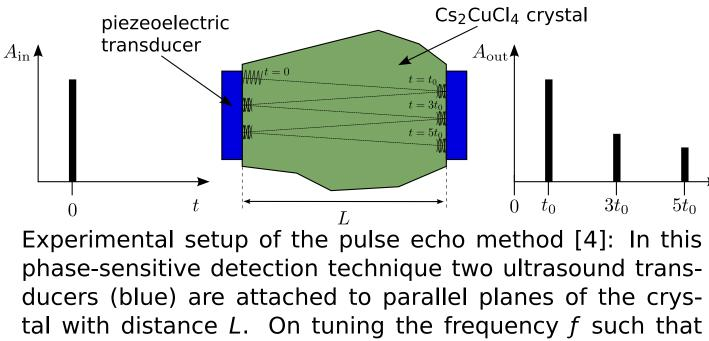
phase-sensitive detection technique two ultrasound transducers (blue) are attached to parallel planes of the crystal with distance L. On tuning the frequency f such that the echo signal remains unchanged one can measure the change of the sound velocity  $dc_{\lambda}/c_{\lambda} = df/f$  and the relative attenuation rate  $\Delta \alpha \propto 1/L \ln(A_1/A_0)$  simultaneously.
