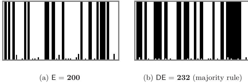
Figure 2: Sequential space-time diagrams for rules E et DE and n = 100 . Time goes from bottom to top ; we go from one line to another after n iterations (i.e., lines represent states of the automaton for times i \cdot n, i \in \mathbb{N} ). This convention is kept for the rest of the paper.
