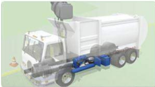
Hybrid electric and hybrid hydraulic truck power: 60% fuel savings
