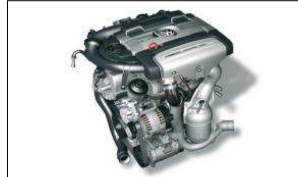
TSI Superchargers for the VW/Audi group: 15% more power, 20% fuel savings
