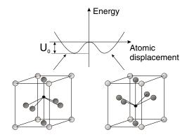
FIG. 1. Schematic of a tetragonal perovskite ferroelectric, characterized by two oppositely polarized ground states, separated by an energy barrier  $U_0$ . For Pb( $Zr_{0.2}Ti_{0.8}$ )O<sub>3</sub>, the corner Pb ions and the center Ti/Zr ions are positively charged, and the face O ions are negatively charged.
