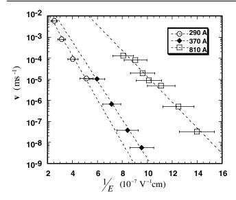
FIG. 3. Domain wall speed as a function of the inverse applied electric field for 290, 370, and 810 Å thick samples. The data fit well to  $v \sim \exp[-\frac{R}{k_B T}(\frac{E_0}{E})^{\mu}]$  with  $\mu = 1$ , characteristic of a creep process.
