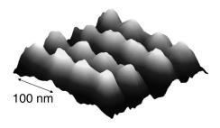
FIG. 4. Piezoelectrically imaged high-density ferroelectric domain array at 28 Gbit/cm<sup>2</sup>, written with 500 ns pulses.
