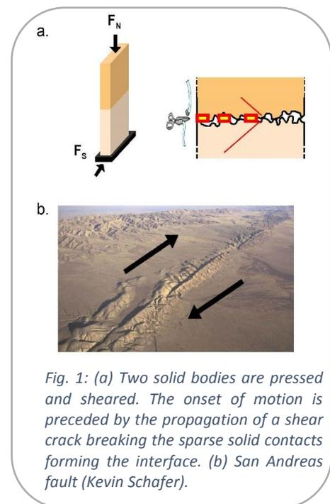
Fig. 1: (a) Two solid bodies are pressed and sheared. The onset of motion is preceded by the propagation of a shear crack breaking the sparse solid contacts forming the interface. (b) San Andreas fault (Kevin Schafer).
