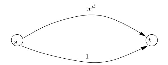
Figure 3: The price of anarchy can be arbitrarily high. Traffic rate is 1. The figure shows latency mappings for both edges. In Nash equilibrium all flow goes through the upper edge. Calculate the optimal flow.
