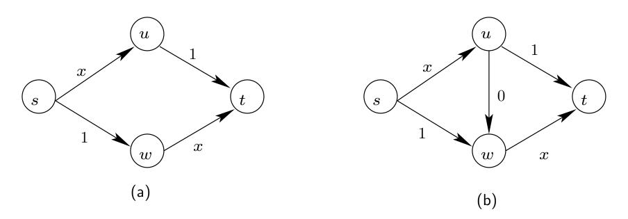
Figure 2: The traffic rate is 1. Latency functions are the same as in the previous example. In (b) the latency on (u, w) edge is 0.
