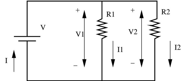
$$V1 = I1 * R1 \wedge V2 = I2 * R2 \wedge V - V1 = 0 \wedge V - V2 = 0 \wedge V1 - V2 = 0 \wedge I - I1 - I2 = 0 \wedge -I + I1 + I2 = 0$$
