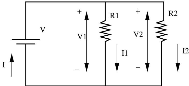
$$V1 = I1 * R1 \wedge V2 = I2 * R2 \wedge V - V1 = 0 \wedge V - V2 = 0 \wedge \\ V1 - V2 = 0 \wedge I - I1 - I2 = 0 \wedge -I + I1 + I2 = 0 \wedge R1 = 5 \wedge R2 = 10$$
