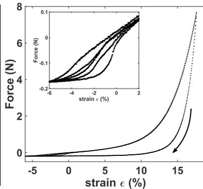
**Legend:** Picture of the deformed stockinette-knit fabric (left). Mechanical response of the fabric over 5 loading–unloading cycles (right).
