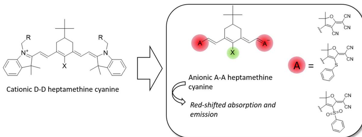
Figure 2. D-D heptamethine cyanine, targeted A-A heptamethine cyanine with the new electron-acceptor groups.
