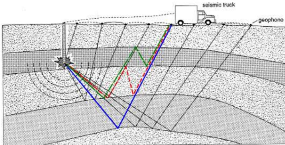
Figure 5: Seismic data acquisition: focus on multiple reflections
