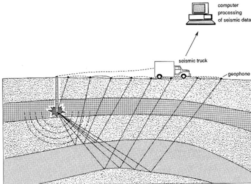
Figure 2: Seismic data acquisition and wave fields
