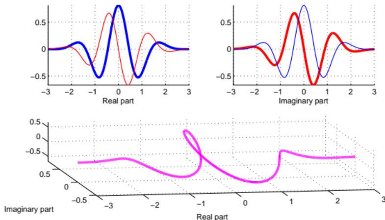
Figure 10: Complex wavelets at two different scales — 1
