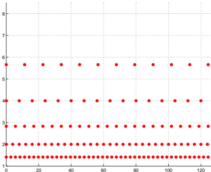
Figure 15: Wavelet frame sampling:  $J = 5$ ,  $b_0 = 2$ ,  $a_0 = \sqrt{2}$
