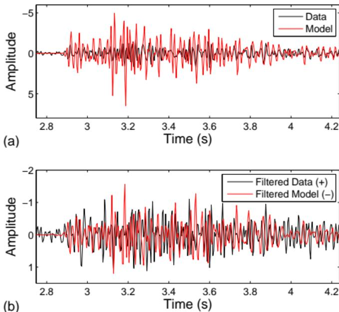
Figure 7: Multiple reflections: data trace, template and adaptation
