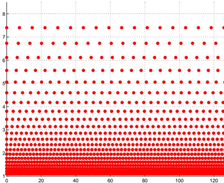
Figure 15: Wavelet frame sampling:  $J = 21$ ,  $b_0 = 1$ ,  $a_0 = 1.1$
