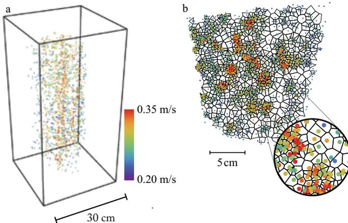
**Legend:** (a) 3D reconstruction of 2mm glass spheres settling in water, colored by their velocities. (b) Top view of fig.(a) showing Voronoi tessellation, which emphasizes the column formation.
