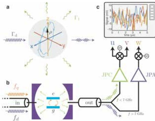
**Legend:** *a.* One observed quantum trajectory followed by a superconducting qubit. *b.* Scheme of the setup that intercepts both spontaneous emission and dephasing signals. *c.* A single measurement record leads to the trajectory in *a.*
