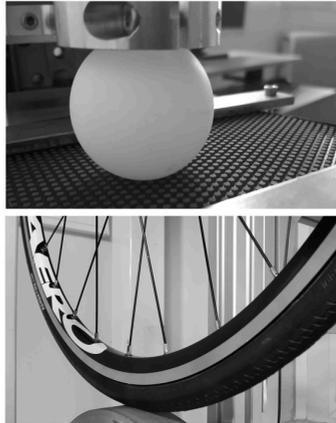
**Legend:** Logo of the Sciences<sup>2024</sup> Consortium (left), and snapshots of experiments studying the rebound of a tennis table ball (top right), and the friction of a wheelchair tire (bottom right).
