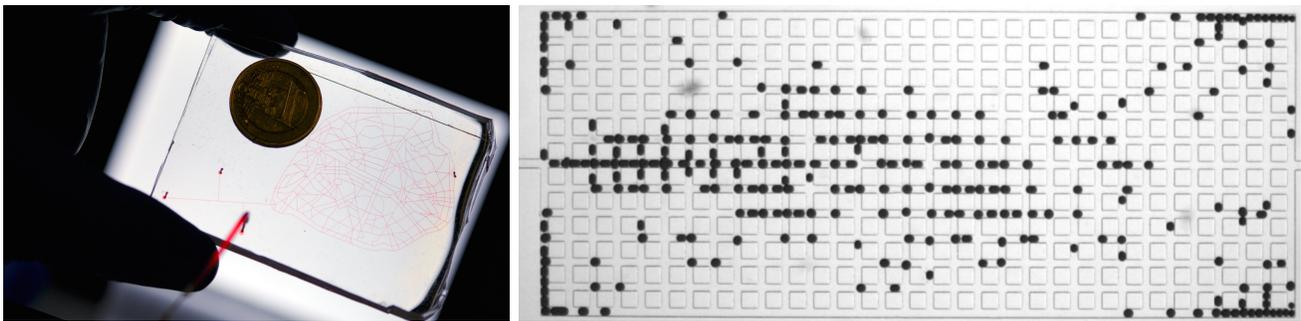
FIGURE 1 – Two microfluidic networks Left : The network geometry is that of the Paris street map. Right : Traffic of emulsion droplets drive through a periodic lattice of channels. Channel width  $50 \mu\text{m}$ .
