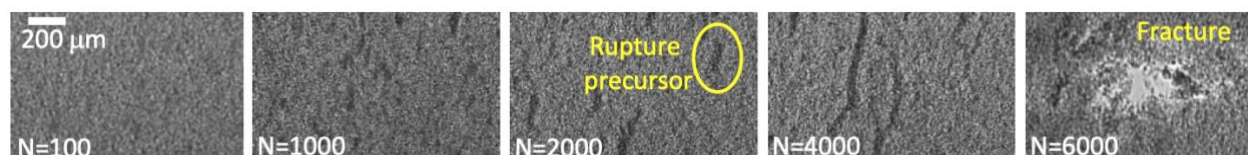
Successive bright-field microscopy images of a protein gel damaged by accumulation of N strain oscillations of amplitude 80%.
