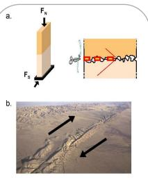
Fig. 1: (a) Two solid bodies are pressed and sheared. The onset of motion is preceded by the propagation of a shear crack breaking the sparse solid contacts forming the interface. (b) San Andreas fault (Kevin Schafer).
