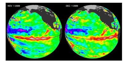
Figure 1: Propagation of an equatorially trapped temperature anomaly before an El Nino event. This is now understood as a topological wave [*P. Delplace, B. Marston, A. Venaille* 2017, Science.]
