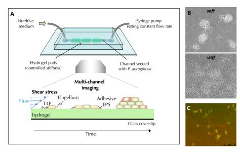
Figure: A. schematic of the experimental setup for in situ imaging of biofilm formation. B. Phase-contrast image of bacteria after 10h on a soft (3 kPa) or a stiff (70 kPa) hydrogel. C. Live staining reveals EPS trails deposited by motile bacteria on a stiff substrate  $\sim 1h$  after attachment.
