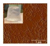
Gel made of cellulose nanofibers and its structure as seen under an atomic force microscope.
