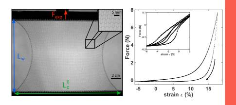
**Legend:** Picture of the deformed stockinette-knit fabric (left). Mechanical response of the fabric over 5 loading–unloading cycles (right).
