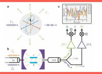
**Legend:** *a.* One observed quantum trajectory followed by a superconducting qubit. *b.* Scheme of the setup that intercepts both spontaneous emission and dephasing signals. *c.* A single measurement record leads to the trajectory in a.
