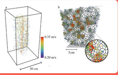
**Legend:** (a) 3D reconstruction of 2mm glass spheres settling in water, colored by their velocities. (b) Top view of fig.(a) showing Voronoï tessellation, which emphasizes the column formation.
